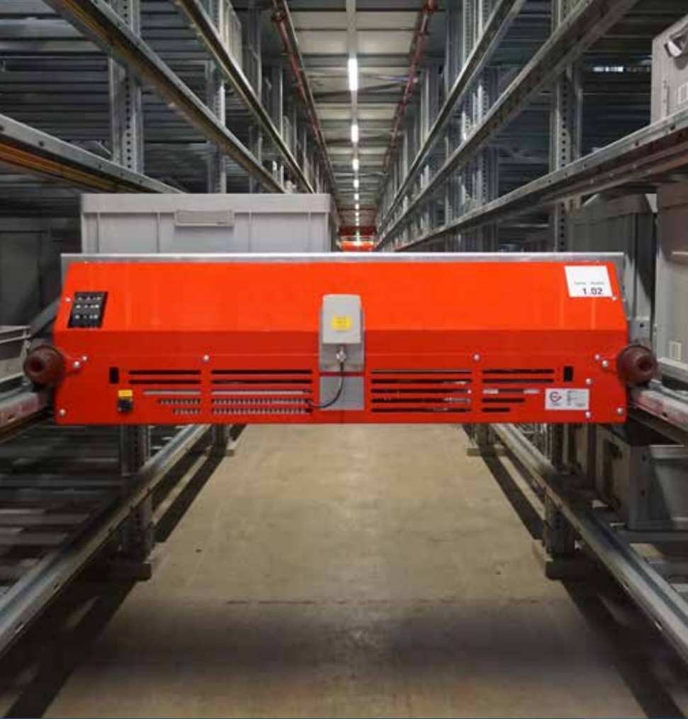
Automatic shuttle system - Double deep | 19,800 box positions
