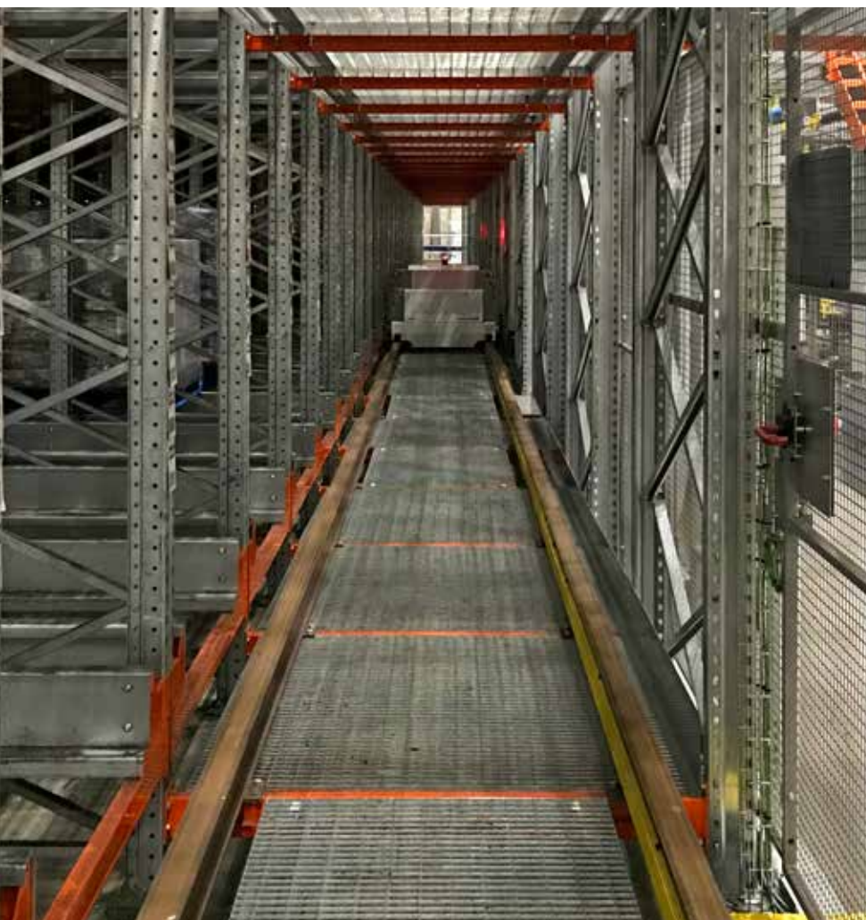
Automated pallet shuttle | 16,000 pallet positions
