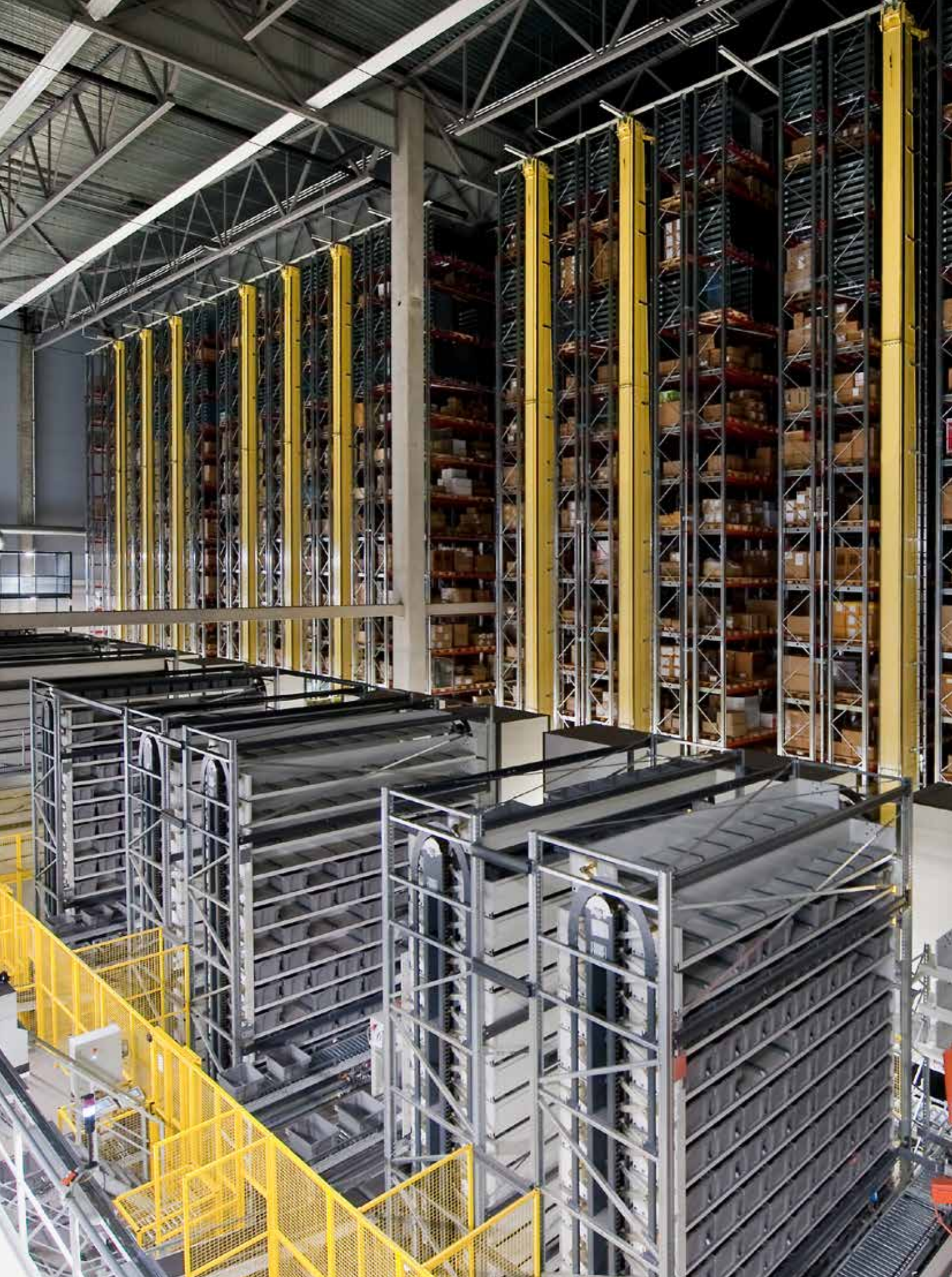
Crane racking & Storage machines | 55,000 pallet positions | 32 paternosters
